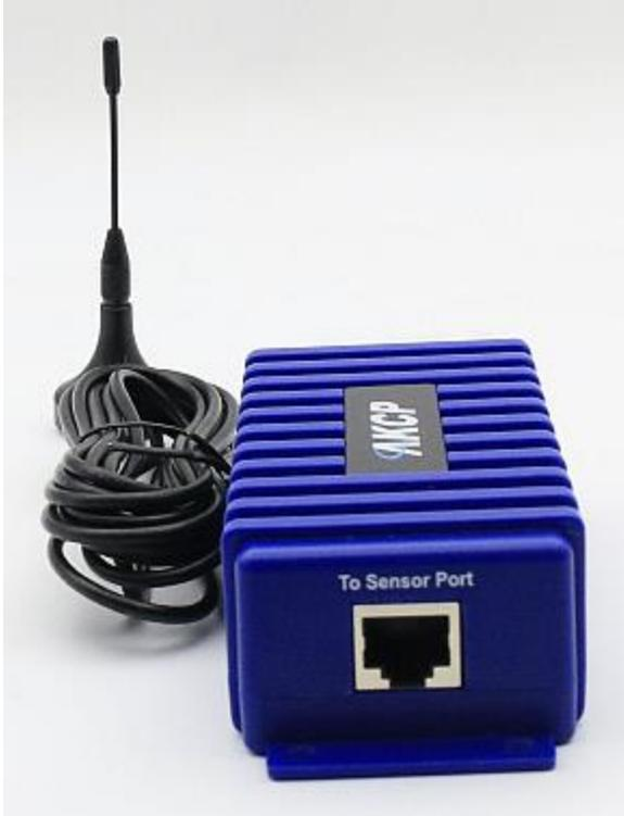
For SPXN units, you just need to plug the modem to the Ext. Modem port and reboot the SPXN; there is no need to set up any options on the WebUI.
