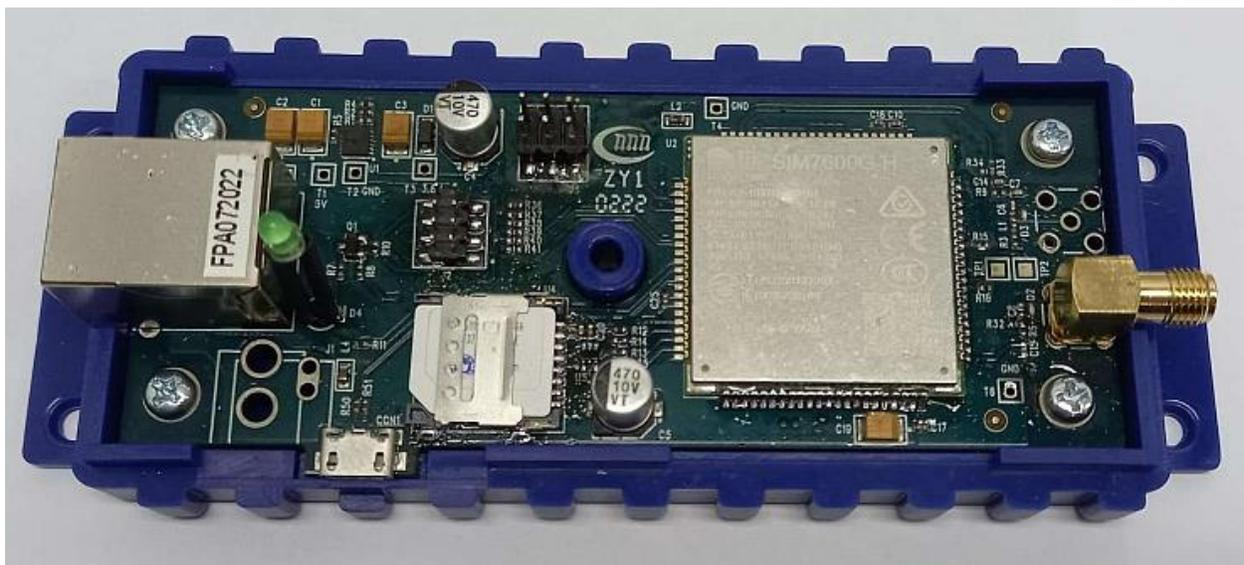
Re-assemble the modem case and connect the GSM antenna to the modem, as shown on the picture below.
