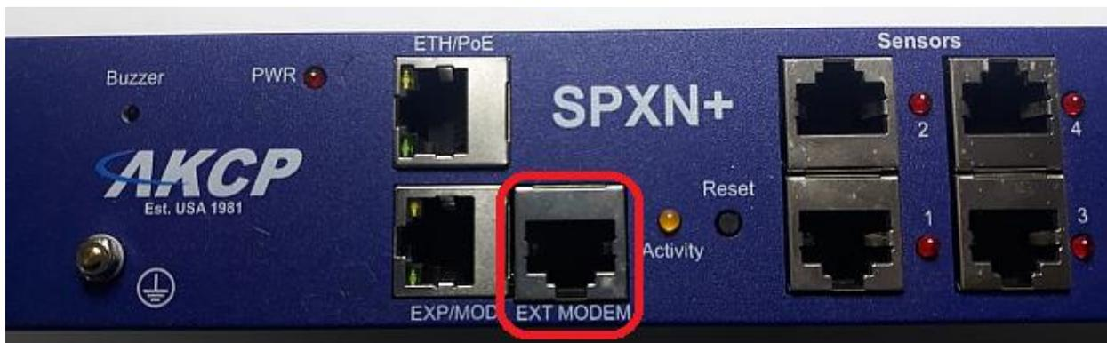
**Important note:** the maximum allowed length of the cable is 12 inches (305 mm).
